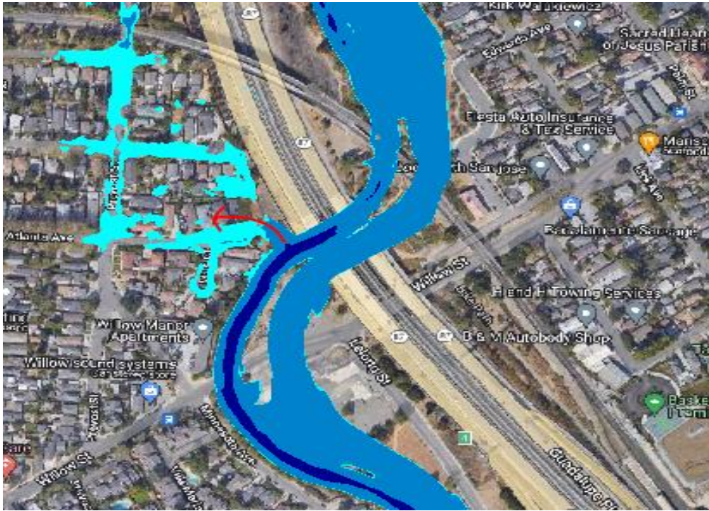
Figure 1: Overbanking on Guadalupe River u/s CA-87
