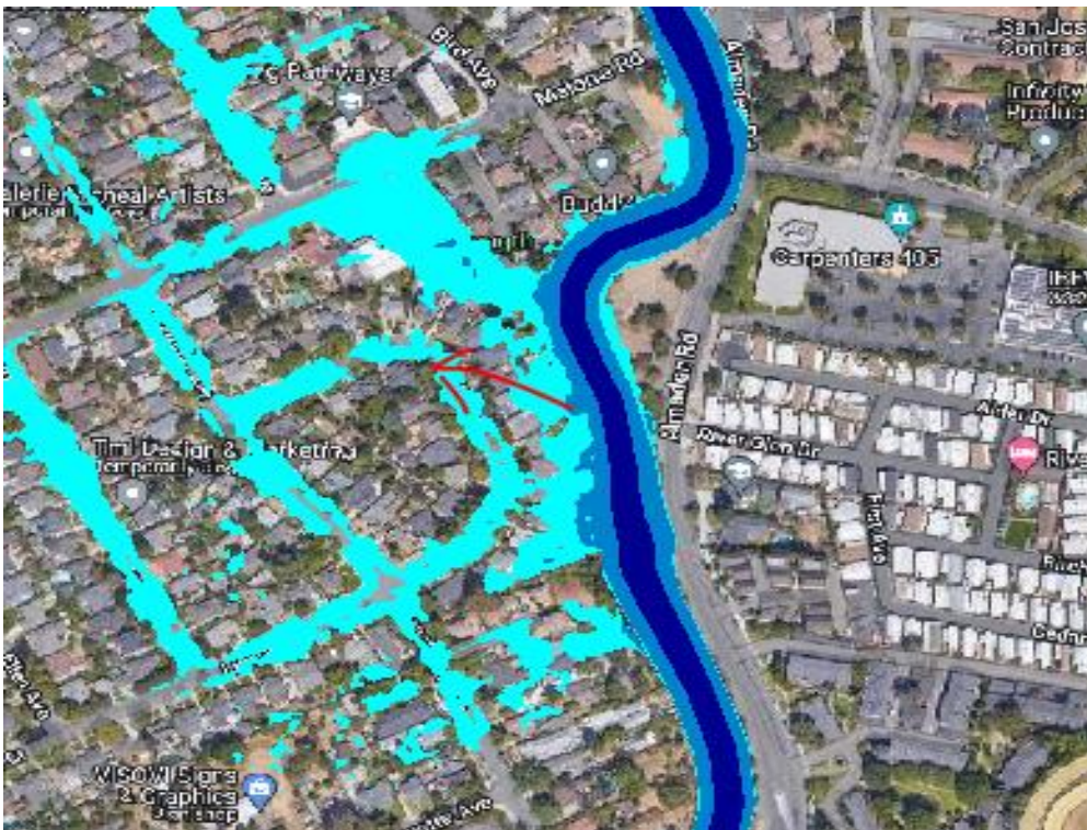
Figure 5: Overbanking on Guadalupe River u/s Malone Road (50 & 100-year)
